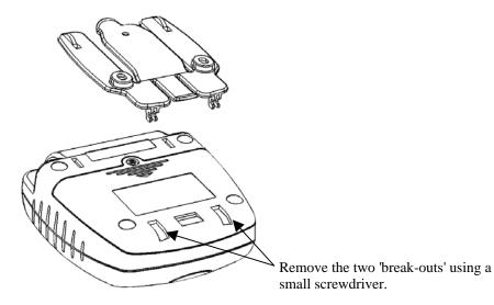
When attaching to a wall, the bracket must be located on the wall using screws and wall plugs as shown. The printer may then be clipped into place and removed as required.
