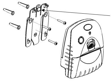
Use a finger or small screwdriver to release the clip and then gently lift the printer to remove from the wall bracket.
